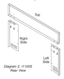
Attach the assembled faceplate to the faceplate mounting brackets.
